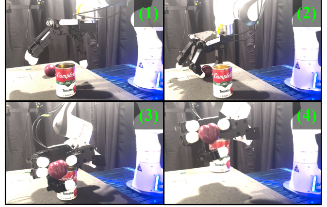
Fig. 1: Overview of SeqMultiGrasp in action using a Franka Panda robot arm and a four-fingered Allegro Hand. From an initial scene with two objects (1), our method first enables grasping and lifting the first object (a fake plum) with two fingers (2). Then, the hand rotates so that it can grasp (3) and lift (4) the can, without losing control of the plum.
